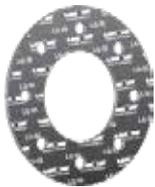
**LG-SS** is a flat metal 316/316L stainless steel reinforced flexible graphite sheet material made with minimum 98% typical carbon content.
