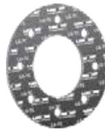
**LG-TC** is a reinforced flexible graphite sheet material laminated with tanged 316/316L stain-less steel insert and made with minimum 98% typical carbon content.
